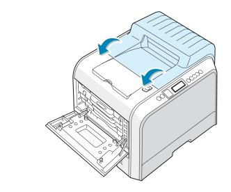
**CAUTION**: Do not try to close the left cover with the top cover open. This may cause damage to the printer.
